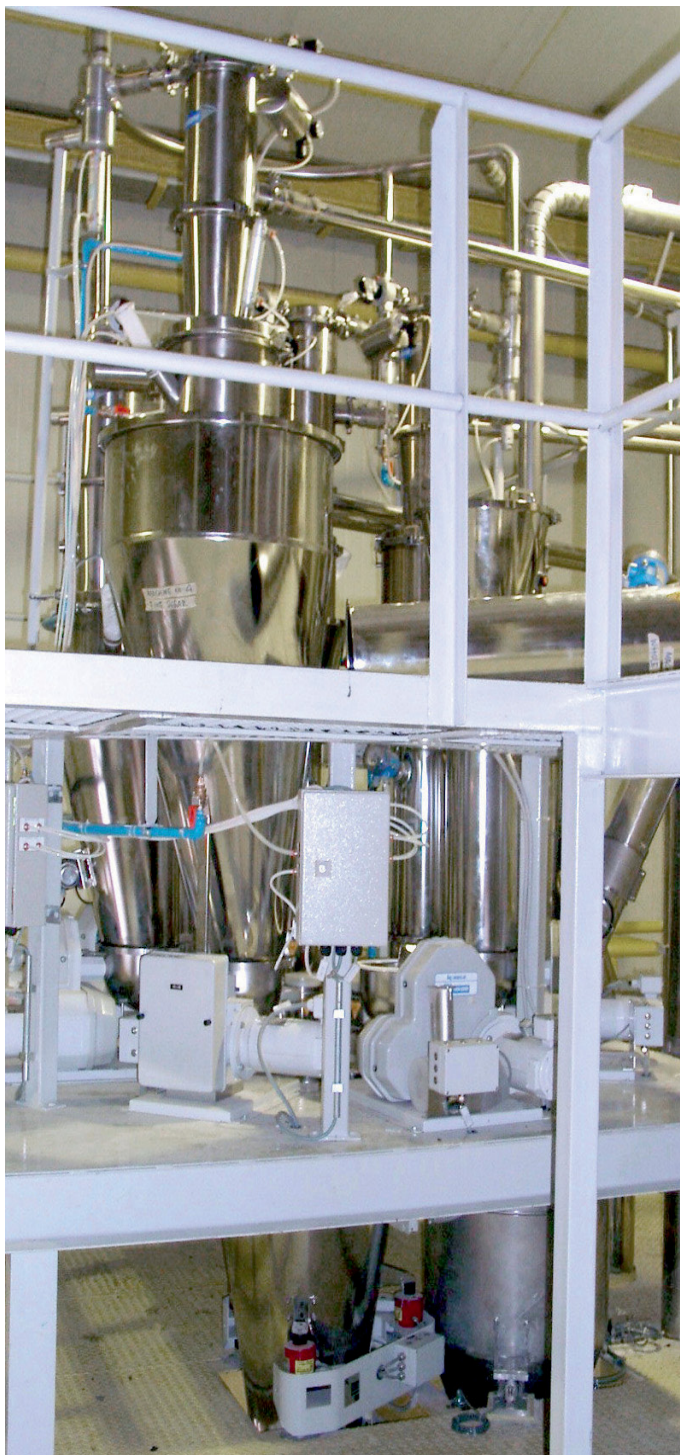
Gain-in-Weight batching station for a bakery installation
